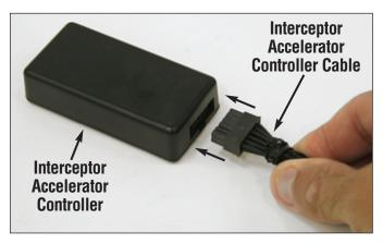
Plug the Interceptor Accelerator Controller cable into the Accelerator Controller as shown above.
