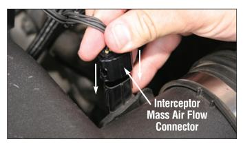
Plug the Interceptor Mass Air Flow sensor connector into the vehicle Mass Air Flow sensor.
