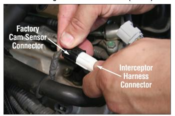
Plug the Interceptor harness connector into the factory Cam sensor connector.
