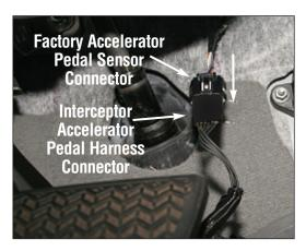
Plug the Interceptor accelerator pedal harness connector into the vehicle's factory accelerator pedal sensor connector.
