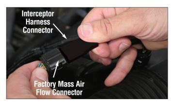
Plug the Interceptor harness connector into the factory Mass Air Flow connector.
