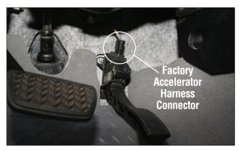
Using a flashlight, locate the factory accelerator harness connector under the driver's dashboard and above the accelerator pedal. Disconnect the factory harness from the accelerator pedal sensor by pushing down on the connector, squeezing the release tab firmly, then pulling up to remove the connector.
