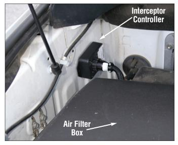
Using the supplied Velcro, attach the Interceptor Controller on the passenger side of the engine compartment as shown above.
