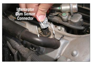
Plug the Interceptor Cam sensor connector into the Cam sensor.
